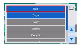
3. Select "Advanced Setting" from Edit and set the "Theta Rotate Type" setting to "Rotate Both".
